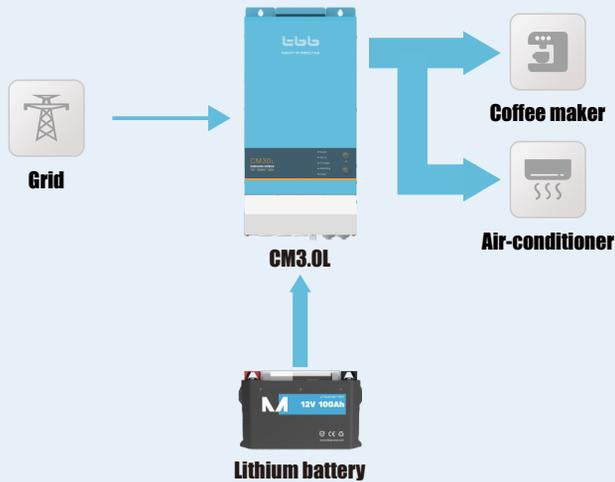
Upon load power exceeding generator capability or limit of AC supply at campsite, Kinergie Mobile could discharge the battery supplying the load in parallel with generator or shore power. Smaller generator or limited AC supply will be capable of handling big load, especially for inductive load which need high surge.
