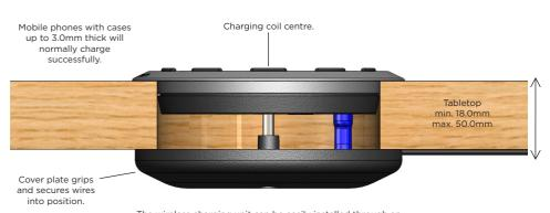
The wireless charging unit can be easily installed through an Ø80.0mm hole in any flat surface. Cables are secured by the retaining plates completing the installation.
