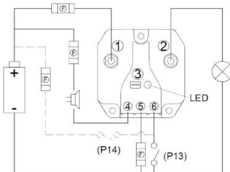
The battery feeds the input of the unit through a fuse on pin 1. The load is connected to 2. The ground line is connected via a 1A fuse to 5. Grounding of pin 6 is an optional override shutdown, while pin 4 provides an optional alarm output.
